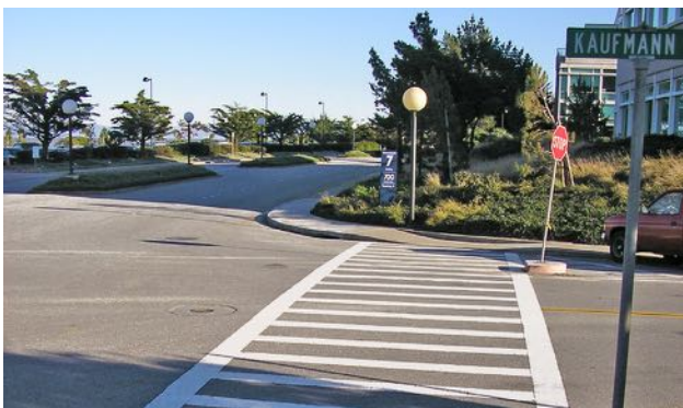
View of Typical Type I Crosswalk at uncontrolled stop. Typical Type II Crosswalks will have similar striping with in-ground flashers.
