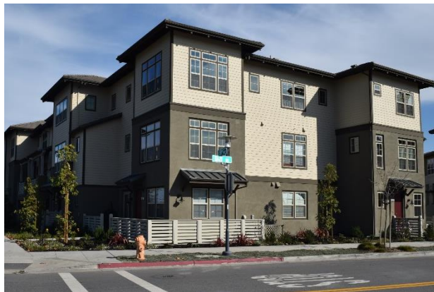
Street-facing building articulation with material and color changes, wall modulations, and awnings.
